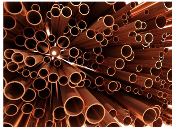
C106: readily welded and brazed for tubes
