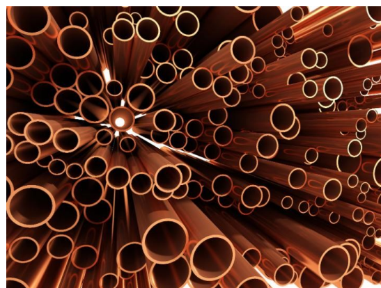
C106: readily welded and brazed for tubes
